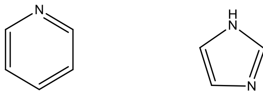
Figure B.16. Structures of bases used in Karl Fischer Titration: Pyridine (left) and Imidazole (right)
