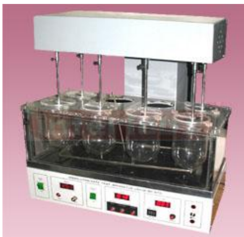
Figure 8-2: Digital Dissolution Test Apparatus (Six Stage) (5)
