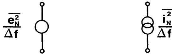
Fig. 3.10: Noise represented by power spectra. a) Noise voltage source, b) Noise current source
