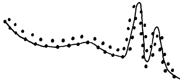
Fig. 6.10: ^{60}\text{Co} spectrum distorted by an ADC with even-odd effect.
