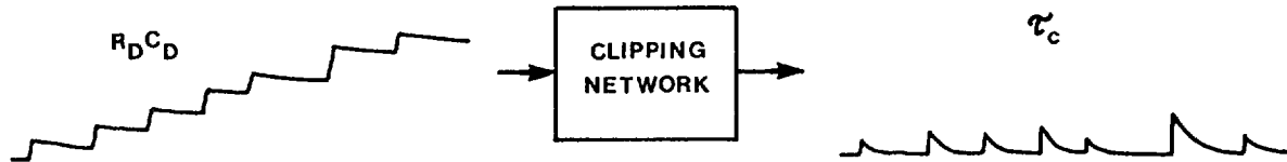
Fig. 1.5: Effect of clipping on the waveform arising from overlapping pulses
