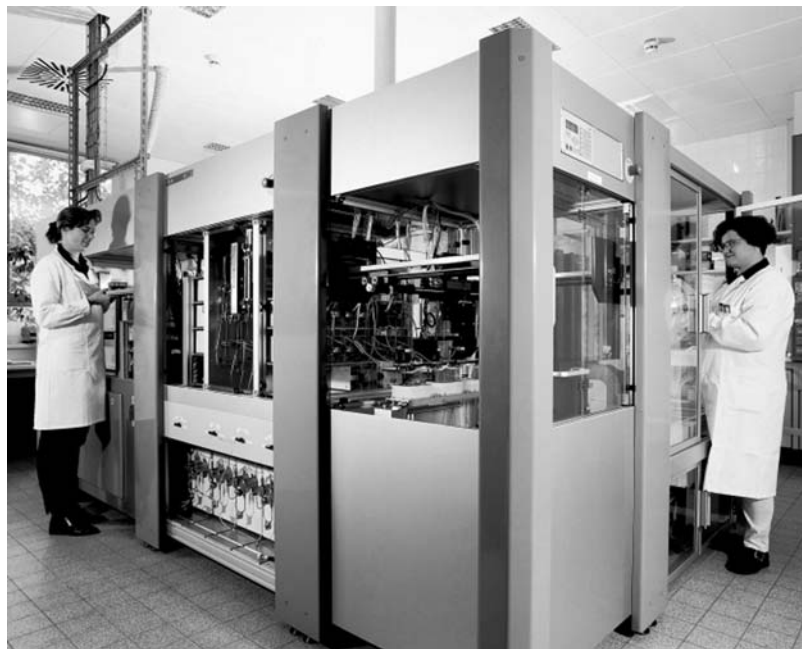
Figure 12.9. Parallel HPLC device for fully automated high-throughput fractionation and purification of natural product extracts on a large scale.
