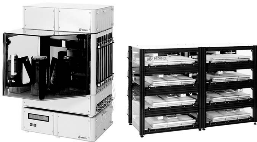
Figure 12.1. Parallel HPLC device ( left ) with flow control unit ( bottom ), autosampler, injection valves, separation columns ( middle ), multiplex photodiode array detector ( top ), and fraction collector ( right ) for parallel fraction collection into 8 \times 12 = 96 microtiterplates.
