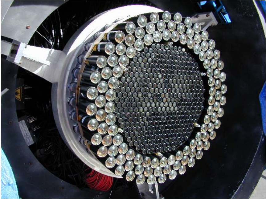
Figure 2.10. The 490 pixel camera of the Whipple Observatory made up of individual photomultipliers. The 379 inner pixels each subtend an angle of 0.12^\circ ; the 111 outer pixels each subtend an angle of 0.25^\circ .
