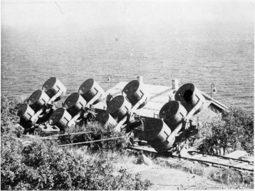
Figure 1.2. The Lebedev Institute experiment that operated in the Crimea, c. 1960–64. This was the first major VHE gamma-ray telescope. (Photo: N A Porter.)
