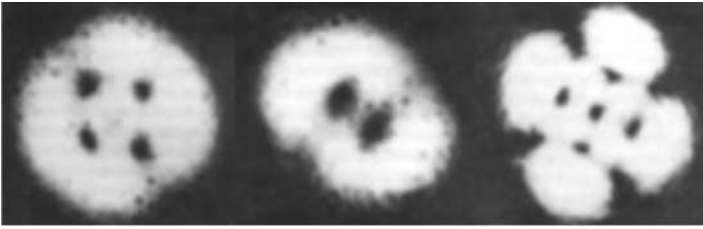
Fig. 6.4. Mode-locked patterns: vortex quadrupole ( left ) and a vortex quadrupole that has degenerated into two vortices of the same charge ( middle ). Both of these plots belong to the mode family 2p + l = 2 . The distribution at the right belongs to transverse mode family 2p + l = 3
