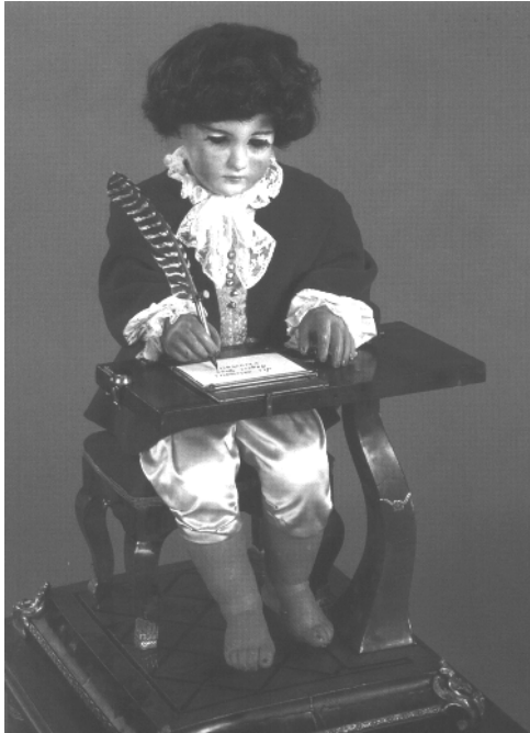
Figure 1.1 The “Writer”, built in the middle of the eighteenth century by the Swiss inventor Pierre Jacquet-Droz, is a beautiful automaton sitting at a writing desk that dips his pen into the inkwell, shakes off the excess ink, and writes Descartes’ famous motto “ Cogito ergo sum. ” The automaton is still fully operational and survives in a Neuchâtel museum.
