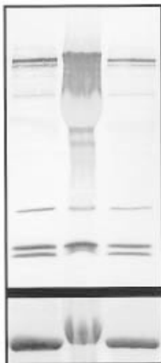
Fig. 7. Distortion in the middle lane of a blot (upper panel) and corresponding gel (lower panel showing myosin band only), caused by contamination of the muscle sample with mountant. The tissue block had previously been oriented for sectioning and the mountant was not removed before the sample was homogenized.
