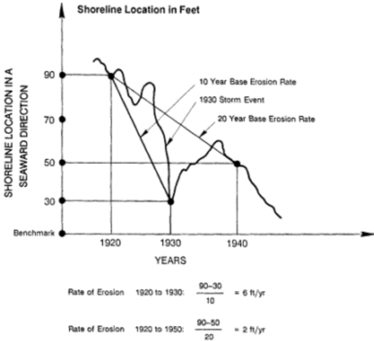
Figure 6-1 Example of the variation of the rate of erosion as a function of the duration of the period of observation, 1920 to 1940.
