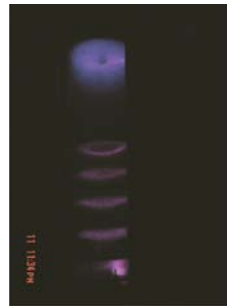
Figure 6. Snapshot photograph of the large glow discharge tube at a pressure of 70 mT (9.2 Pa) and a current density of 0.12 \text{ A/m}^2 illustrating quasi-periodic striations, uniformly distributed across the tube at this pressure.
