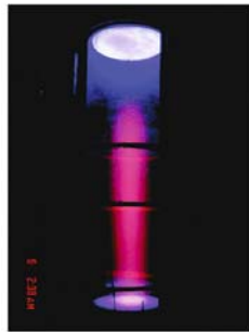
Figure 5. Photograph of the large glow discharge tube at a pressure of 1.2 Torr (160 Pa) and a current density of 6.6 \text{ A/m}^2 . At this pressure, the positive column is restricted relative to the tube diameter.
