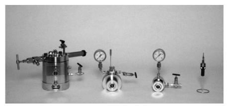
Fig. 2. High pressure reactors and spectroscopic cells as used at the Max-Planck-Institut für Kohlenforschung for exploratory studies on chemical synthesis in  $sccO_2$
