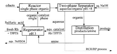
Fig. 9. Catalyst recycling by pH-induced phase separation
