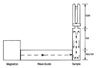
Scheme 25. Dispersion energy in a monomode reactor
