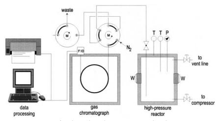
**Fig. 3.** Reactor system for chemical synthesis in  $scCO_2$  with online GC monitoring. T = thermocouple; P = pressure transducer; W = thick-walled glass window. The ports "to vent line" and "to compressor" can be used for addition of  $CO_2$  or other components and for additional sampling
