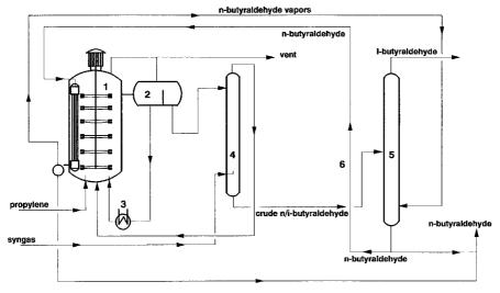
Fig. 6. Flow diagram of the RCH/RP process [27e]
