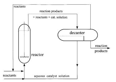
**Fig. 1.** Biphasic concept: the reactor (*left*) is supplied with the reactants; in the phase separator (*right*), the reaction products and the catalyst phase are separated. The catalyst phase is returned by a short route to the reactor
