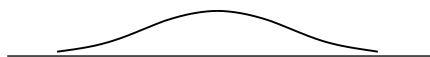
Figure 4-13 The Potential Energy Form Given by the V_{n=1} Term in the Truncated Fourier Series (Eq. 4-21).
