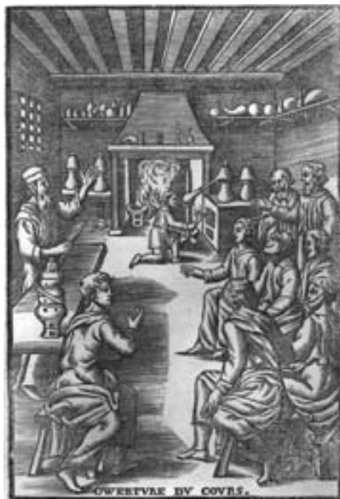
Figure 2.2 Woodcut print of chemical lecture from 1653. Small furnace sits on table and various glassware used for distillation rests on shelves above stove in background. Image from Edgar Fahs Smith Collection, University of Pennsylvania Library.
