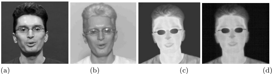
Figure 6.2. A face simultaneously imaged in the (a) visible spectrum, 0.4–0.7 \mu\text{m} , (b) shortwave infrared, 0.9–1.7 \mu\text{m} , (c) midwave infrared, 3.0–5.0 \mu\text{m} , and (d) longwave infrared, 8.0–14.0 \mu\text{m} .
