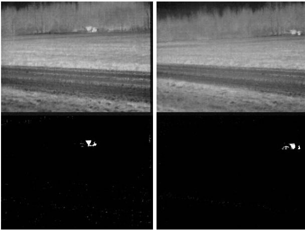
Figure 5.2. Frames 160 and 250 of a moving vehicle IR sequence along with detected objects (sensor recovering after panning motion).
