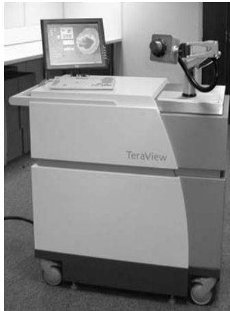
Figure 9.2. The TPI Scan (TM) : A complete terahertz imaging system including near-infrared laser and terahertz imaging optics for imaging biological tissue. Courtesy of TeraView Ltd, Cambridge, UK.
