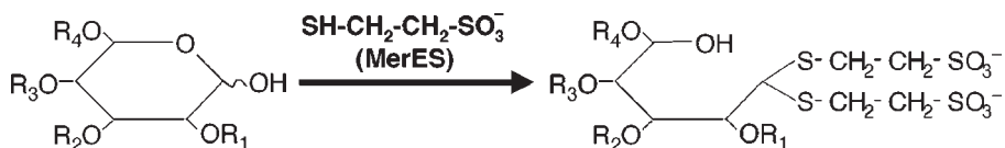
Fig. 1. Introduction of the sulfonate tags to a reducing carbohydrate by dithioacetalation with MerES.
