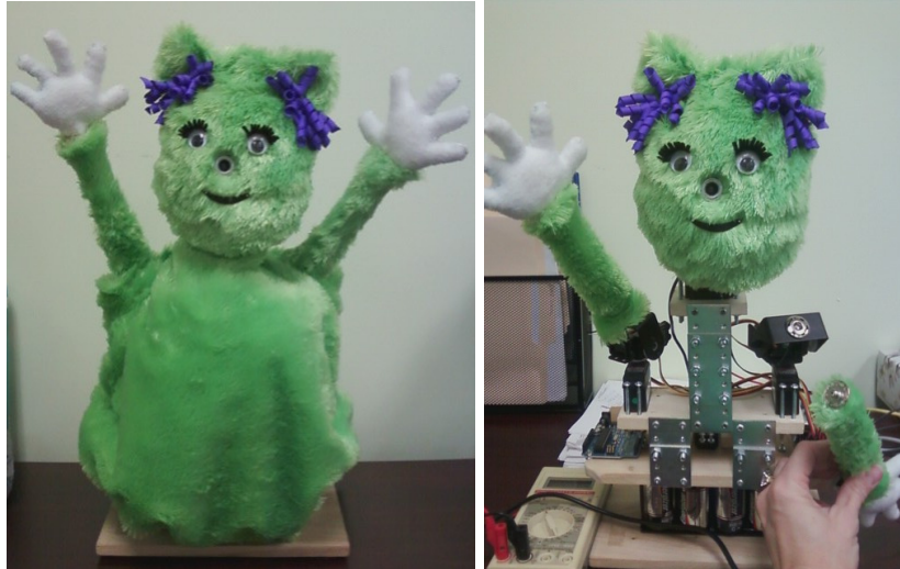
Figure 3.1: CHARLIE. [left] Completed robot. [right] Internal structure.
