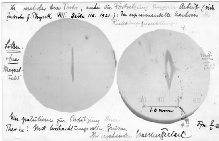
Fig. 5.4 Two figures contained in a letter to Bohr from Stern, communicating his experimental results. Stern explains that the magnetic field was too weak at the extremes of the beam. The figure to the left was obtained, for comparison, in the absence of magnetic field. (Reproduced with permission from Niels Bohr Archive, Copenhagen)
