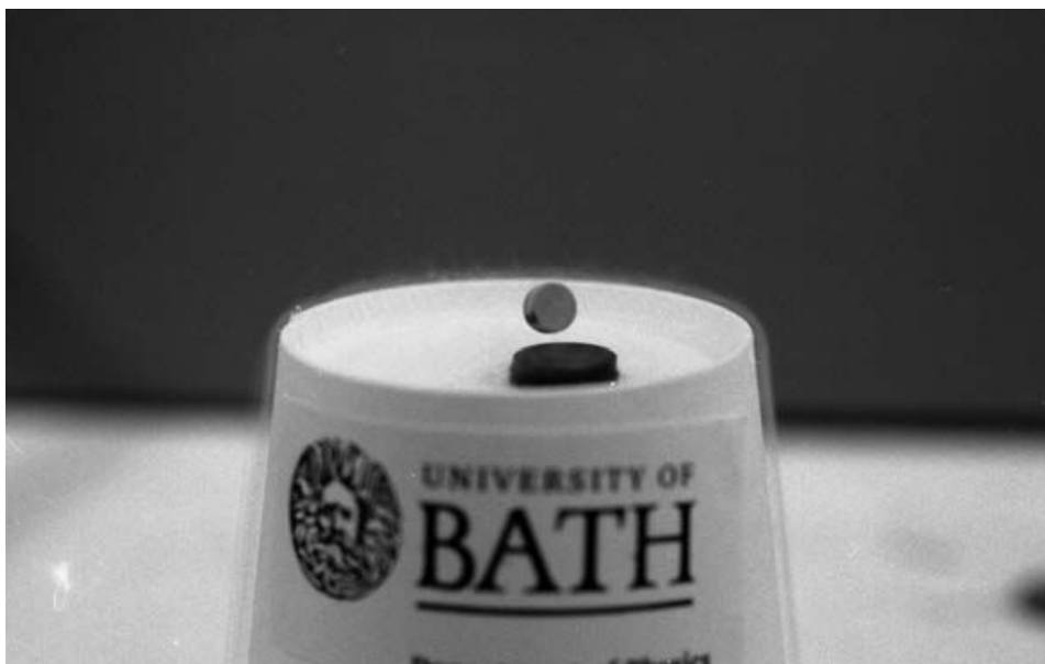
Figure 2.5 Levitation, induced by the persistent surface current and the Meissner effect, of a powerful, small samarium–cobalt permanent magnet above a YBCO polycrystalline sample produced by students in the Department of Physics of the University of Bath.
