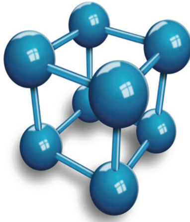
Fig. 3.2. Unit cell of the simple cubic structure. Picture kindly provided by Albin Nilsson
