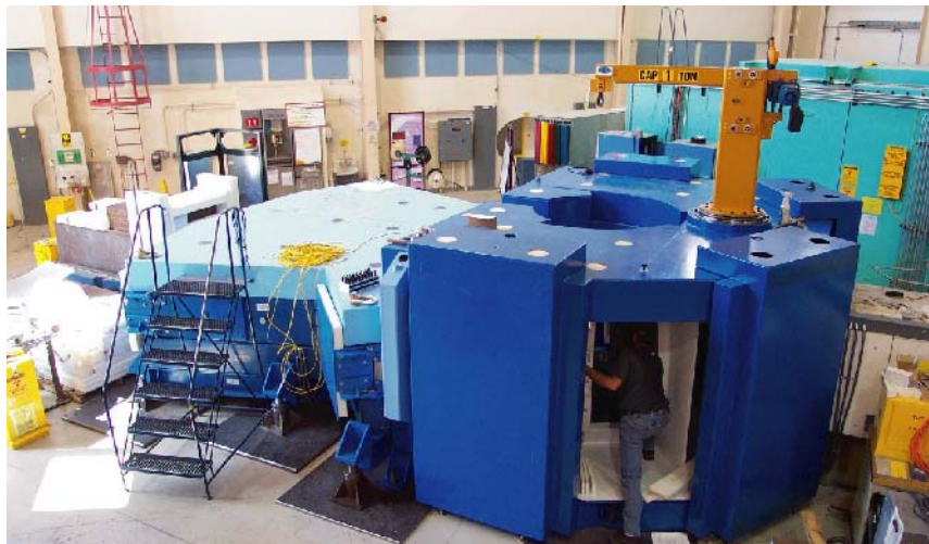
Fig. 5.1. The Neutron Powder Diffractometer (NPDF) of the Lujan Center, Los Alamos National Laboratory, during the upgrading work supported by the National Science Foundation DMR00-76488. A large backscattering detector frame for position-sensitive ^3\text{He} detectors is seen with a technician inside
