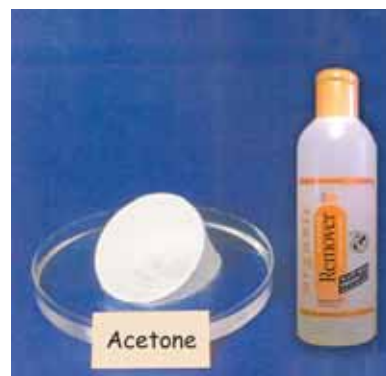
Acetone ( \text{C}_3\text{H}_6\text{O} ), a solvent found in nail polish removers, will quickly dissolve a styrofoam cup.
