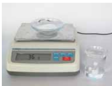
The solubility of table salt ( NaCl ) is 36 g/100 g of water at 20°C.
