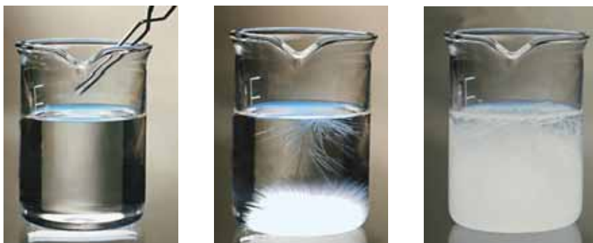
Figure 12 When a small seed crystal of sodium acetate is added to this supersaturated solution, the excess salt quickly crystallizes.
