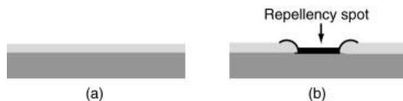
FIGURE 9.5. Even a monolayer of physically adsorbed material can have a disastrous effect on some technological processes, especially critical coating processes in which absolutely smooth, uniform coating is required such as the microelectronics industry. (a) An uncontaminated surface should produce a smooth, uniform coated layer. (b) Surface contamination by a lower-energy material (such as oil molecules) may result in the formation of “repellency” spots or other defects, producing less than optimum or even useless finished products.
