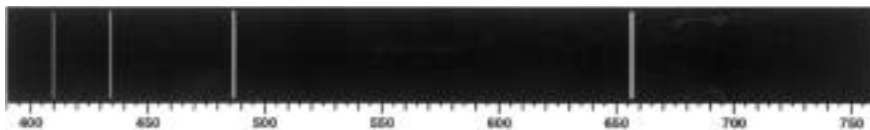
Figure 3.1 The visible spectrum of hydrogen, called the Balmer series. The wavelengths of these spectral lines are, from left to right, 4,101.2 Å, 4,340.1 Å, 4,860.74 Å, and 6,562.10 Å.
