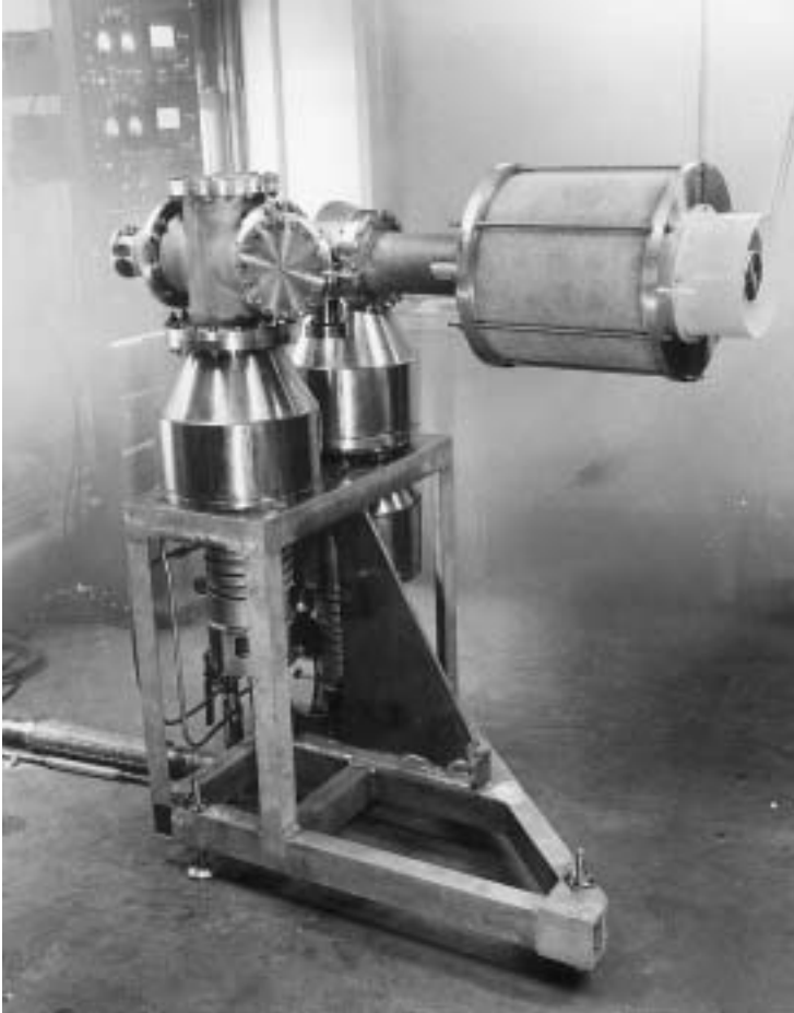
Figure 18.2 The early hydrogen maser, forerunner of the hydrogen maser clock.
