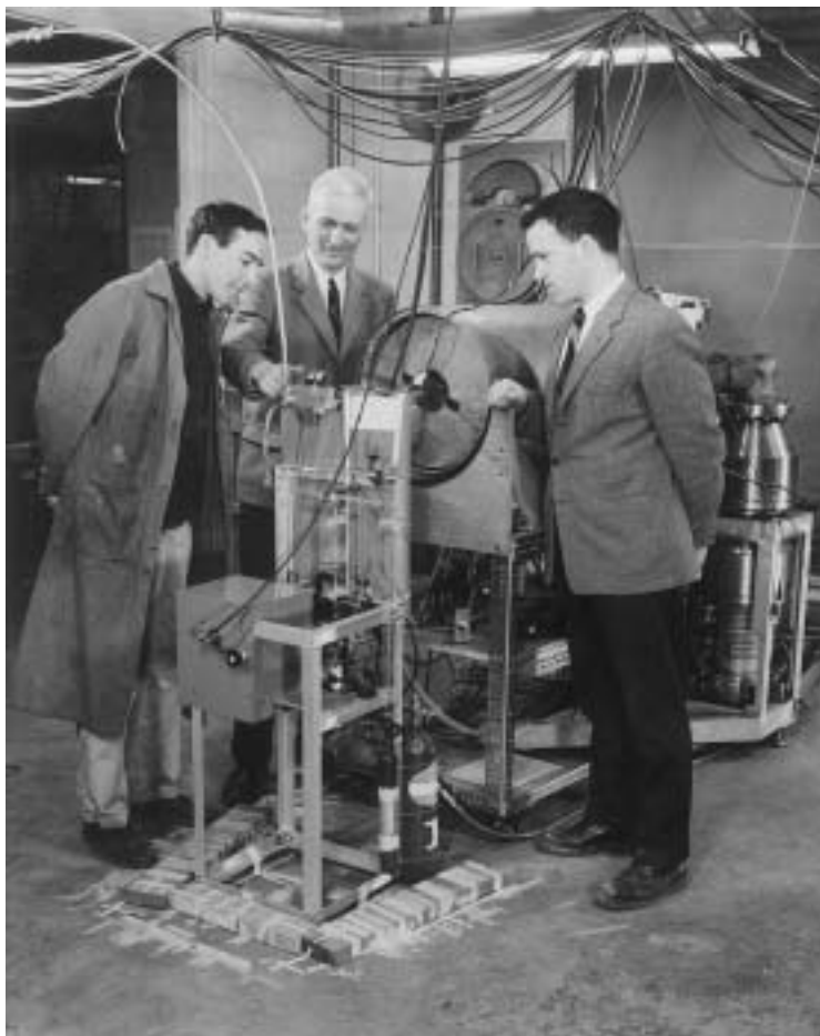
Figure 18.1 Norman Ramsey ( center ), Daniel Kleppner ( right ), and another Ramsey graduate student, Stuart B. Crampton, standing beside a version of the hydrogen maser clock.
