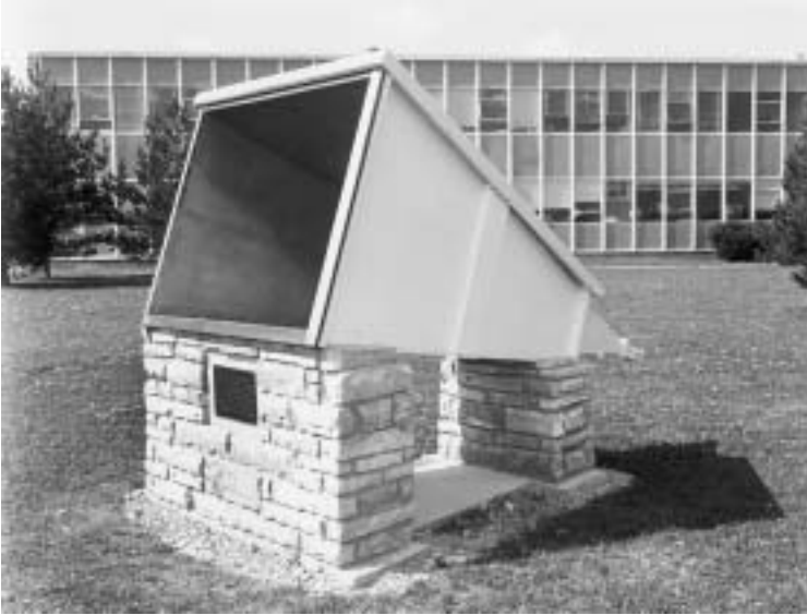
Figure 17.2 The horn antenna used by Purcell and Ewen in their discovery of the hydrogen 21-cm line.
