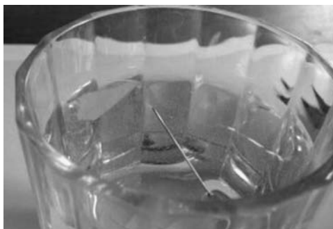
FIGURE 1.4 An iron needle floats on the surface of water ( only if carefully placed; otherwise, it should sink due to gravity forces ).
