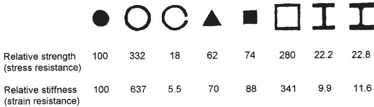
Figure 1.33 Relation of cross-sectional geometry to torsional resistance.
