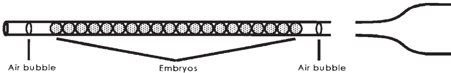
Fig. 2. Transfer pipet. The transfer pipet, connected to a mouthpiece, is used to collect the injected eggs/embryos (about 20 of them). Air bubbles are aspirated before and after the eggs/embryos to serve as a marker during the transfer.
