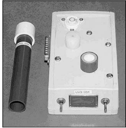
Figure 4.19. UV-A radiometer with optional collimating tube.
