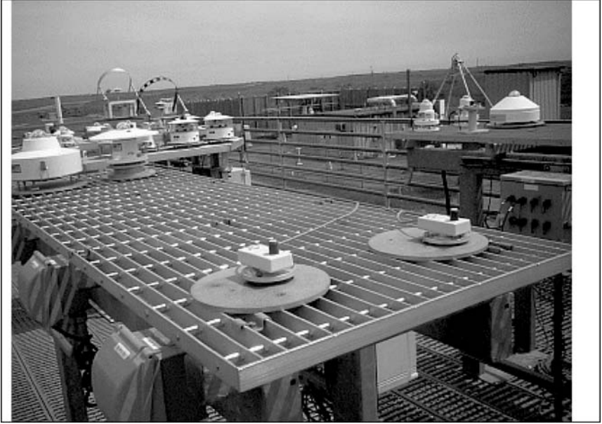
Figure 4.10. PDB-C139 SIPs being calibrated at NREL.
