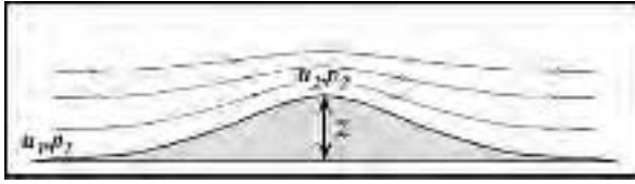
Figure 3.15 Flow over a hill illustrating the effect of dynamic pressure. Thin lines are streamlines of the flow – the closer the streamlines in the vertical, the greater the flow speed. Since u_2 > 0 , p_2 is less than the hydrostatic pressure at height z
