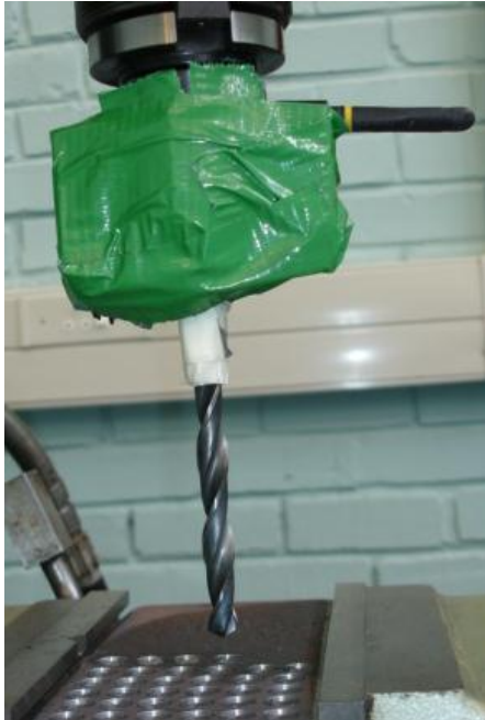
Figure 4.5 and 4.6: Instrumented drill with telemetry transmitter and milling machine equipment
