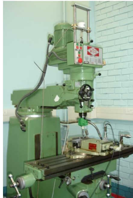
Figure 4.5 and 4.6: Instrumented drill with telemetry transmitter and milling machine equipment
