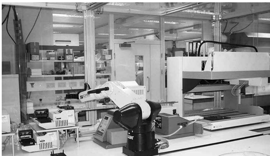
Figure 3 Automated Rhinovirus 3C protease screening robotic system. This system, built by Scitec, is capable of running both cellular and non-cellular 96-well and 384-well assays in a fully automated fashion. Seen here is a CRS robotic arm which runs on a 5 metre linear track and is used for transferring microtitre plates from one piece of equipment to another, two Labsystems Multidrops (one of which was used to add enzyme) and a Matrix Platemate with 96-well head which was used to add substrate solution in neat DMSO. Also visible in this picture, but not used, are a Skatron plate washer and Tecan Genesis liquid handling system. Out of shot but present on the system is a Tecan Spectrafluor Plus used to read the fluorescence in the plates. Also the system has a Scitec plate hotel, a plate shaker and a CO 2 incubator, none of which were required for this assay. The whole system is enclosed in a cabinet for safety reasons. This system is designed to be modular, so it would be possible to exchange pieces of equipment with upgraded versions or to add more readers and/or liquid and cell handling devices as required.
