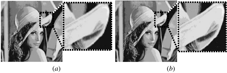
FIGURE 6.6 (a) Low-resolution Lena image containing 3 bits of dynamic range; (b) super resolved reconstruction using gray-level multiplexing.
