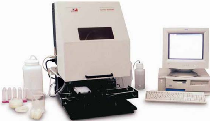
Fig. 1. Picture of the COPAS™ Biosort with the accompanying desktop computer and associated liquid containers.
