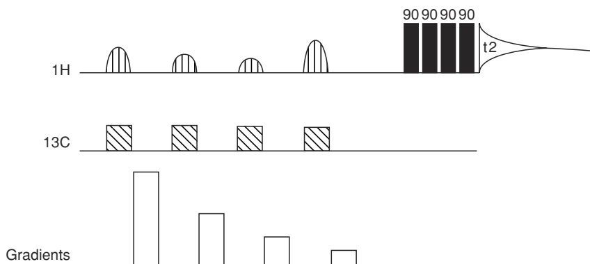
Figure 1.16 Representation of the WET pulse sequence for multiple solvent suppression
