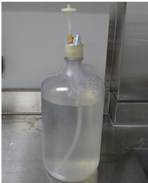
Fig. 5 A small (2") piece of 1/8" tubing is attached to a 0.2 \mu\text{m} syringe filter connected to one of the ventilation ports on the cap of a Nalgene carboy. Inside the cap, 18" of 1/8" tubing is attached to the opposite ventilation port. Cover the uncovered ventilation port with aluminum foil or autoclavable paper and then autoclave
