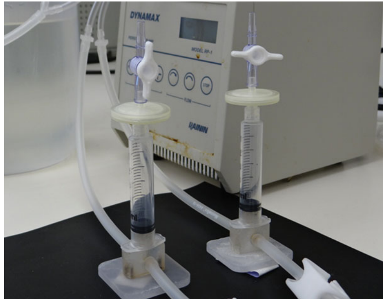
Fig. 6 Attach two 5 ml syringes to two 0.2 \mu\text{m} syringe filters and connect valves to the top of syringe filters. Remove plungers from 5 ml syringes and place on top of bubbles traps. Left valve is shown in “open” position and right valve shown in “closed” position
