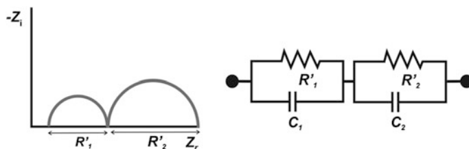
Fig. 3.34 The Nyquist diagram corresponding to a “dual” equivalent circuit describing the charge transfer on the electrode covered with the layer of a finite thickness
