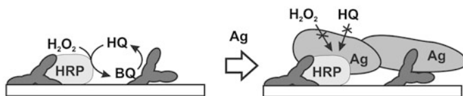
Fig. 2.12 Detection of Ag–Ab formation on the electrode by inhibition of the reaction of enzyme co-immobilized with specific antibodies. HRP horseradish peroxidase, HQ hydroquinone, BQ benzoquinone
