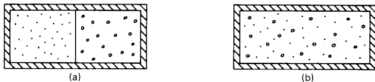
FIGURE 3.14. (a) Confined gases. (b) Gases expand to fill the whole interior region. For mole concentrations, state (a) is not observed to reoccur.
