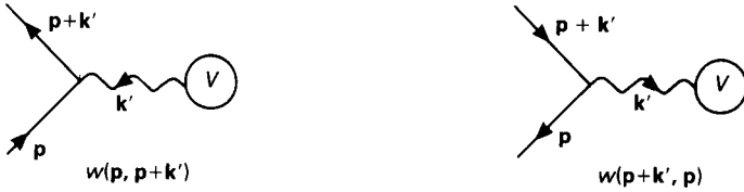
FIGURE 5.3. Diagrams for scattering by the potential V . For elastic interactions, the rate for collision and its reverse are equal.
