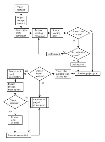
Figure 3.3 Software project planning/project planning flowchart.
