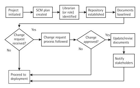
Figure 7.1 SCM/Configuration Management Flowchart
