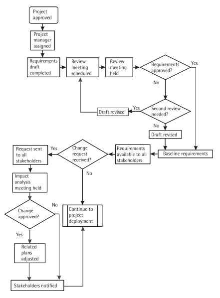
**Figure 2.1** Software requirements management/requirements management flowchart.
