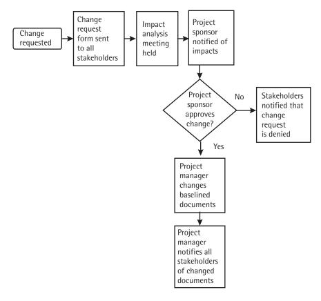
Figure 6.2 Change control procedure.
