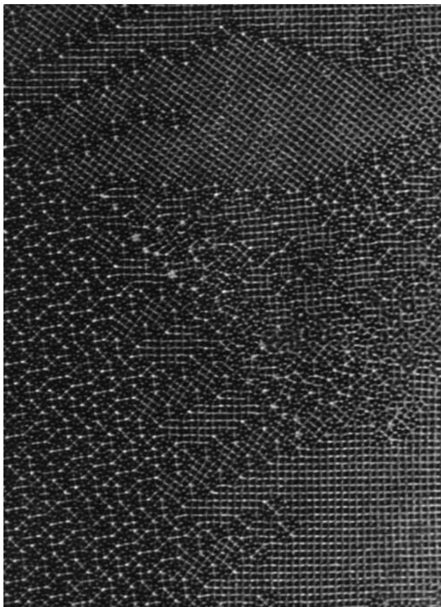
Fig. 13.14 Solid state chemical reactions in action. HREM image along [001] of in-situ oxidation product of \text{Nb}_4\text{W}_{13}\text{O}_{47} , oxidised in an environmental cell under 20 mbar of oxygen. Domains of different structure appear as a result of the oxidation. Microdomains of \text{WO}_3 , tetragonal tungsten bronze and disordered bronze structures can be identified. (Modified JEOL 4000EX.) (See Krumeich et al. (1999).)
