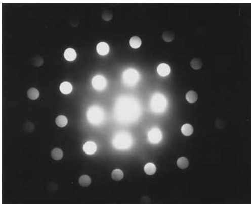
Fig. 12.7 Diffraction pattern from the silicon crystal used to form the images in Fig. 12.4. The condenser lens is fully focused, showing the illumination conditions used when recording the images. The 'beam divergence' can therefore be obtained from a picture such as this (see Section 4.6). The crystal is close to the symmetrical [110] zone-axis orientation (see also Section 5.6).
