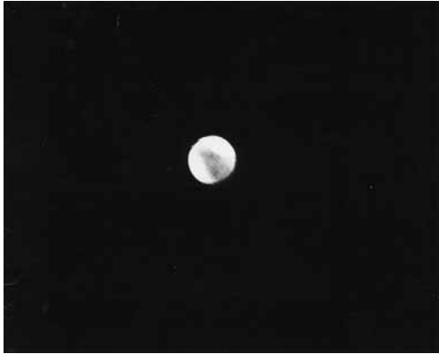
Fig. 12.6 Defocused central diffraction spot from a small triangular-shaped silicon crystal. The out-of-focus diffraction pattern makes each diffraction spot into a low-magnification image of the specimen, allowing simultaneous observation of the crystal orientation and position. As the specimen is tilted, corrections can be made to the translation controls to keep the same region of specimen in view.
