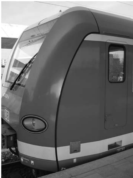
Figure 10.8 Bonded driver's cab – carriage bodywork of a suburban train.
