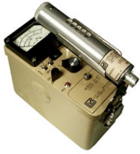
Figure 19. Hand-held survey meter [Ludlum, 2004].
