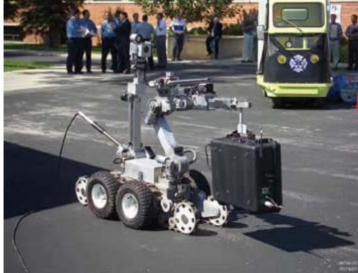
Figure 24. The PIRATE portable WMD analysis platform. The sensors and communication transmitter are installed in the suitcase-like container [KC, 2004].
