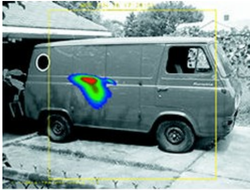
Figure 20. GammaCam TM image of a gamma-ray source inside a truck [EDO, 2004].
