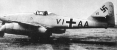
The Me 262A (V1 + 44) with the late model James ballast of the production series aircraft showing the revised cowling panel. Both rudder and trim tab have mass balancers. Note canopy pins and the experimental hydraulic filler point.
