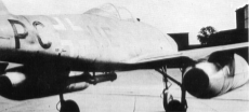
The Me 262 (PC-412) after modification as the prototype underwing layout. The underwing engine doors were locked shut and the main air intakes remained in order the drag as much as possible. Two Borep systems are visible beneath the fuselage. The original shape of the doors.
