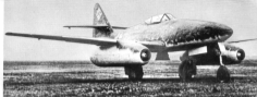
Another My 282A-1a minus bomb racks and showing the upper gear deleted, the recess being covered by dipole fabric.
