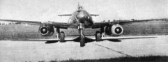
The dorsal triangular shape of the fuselage is well shown in this view. The port engine is a replacement, hence the difference in coloring.
