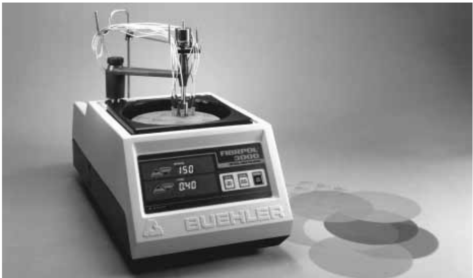
Figure 6-7 Automatic polishers can polish large quantities of connectors quickly. Courtesy Buehler LTD
