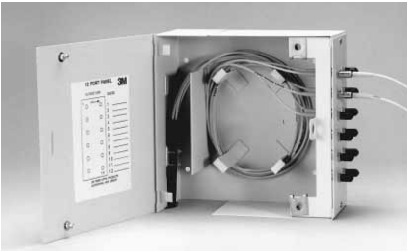
Figure 7-4 The patch panel makes connection between two cables. Here we see single fiber jumpers connected to a breakout cable. Courtesy 3M
