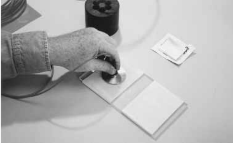
Figure 6-6 A polishing puck holds the connector properly for polishing.
