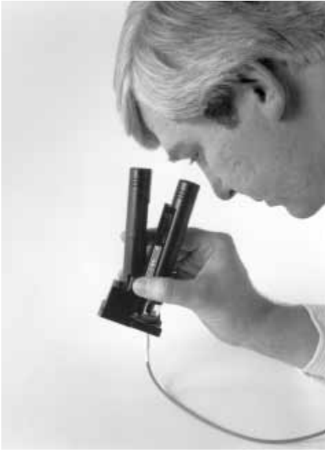
Figure 17-6 Microscopes allow inspection of connectors for polish quality, cleanliness, and faults. Courtesy Fotec, Inc.
