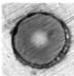
TYPICAL 1 MICRON FINISH AT 200X
