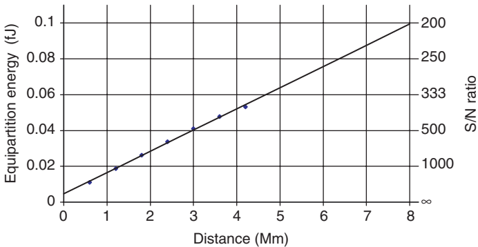
FIGURE 3.12 Experimentally measured noise as a function of distance for the loop of Fig. 3.11. The S/N ratio indicated by the vertical scale on the right is based on an assumed signal pulse energy of 20 fJ.
