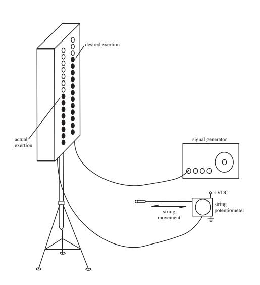
**Figure 1.3:** KNH project overview. A display panel contains two arrays of 14 large (10 mm diameter) red LEDs each. The right array driven by a signal generator indicates the desired assertion level. The left array is driven by a string potentiometer transducer. This LED array indicates the actual exertion level as determined by the string length of the potentiometer.
