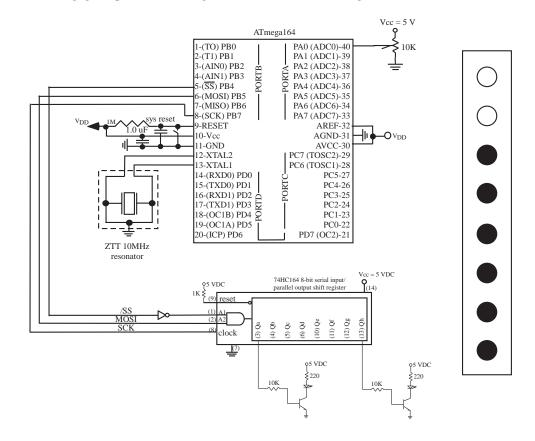
Figure 4.11: ADC with rain gage level indicator implemented via the SPI.
