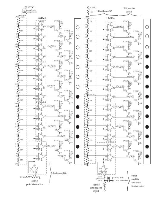
**Figure 1.6:** Circuit diagram for the KNH arrays. (left) Actual exertion array and (right) desired exertion array.
