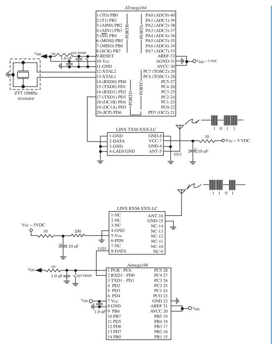
**Figure 3.7:** USART radio frequency link. The "XXX" specifies the operating frequency of the transmitter and receiver modules.
