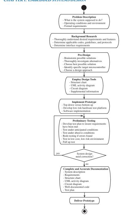
Figure 1.1: Embedded system design process.
