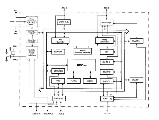
Figure 2.3: Atmel AVR ATmega164 Block Diagram. (Figure used with permission of Atmel, Incorporated.)
