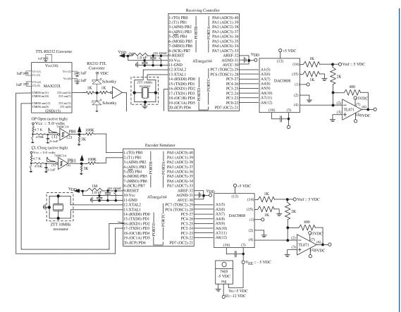
Figure 5.6: Encoder test configuration.
