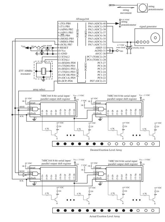
Figure 3.12: KNH arrays implemented with SPI system.
