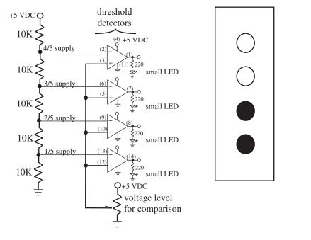
**Figure 1.5:** Small scale test circuit for the KNH arrays. The input voltage is compared against a bank of threshold detectors, each set to a different fraction of the supply voltage. As the input voltage is increased, more LEDs will illuminate. This is commonly referred to as a rain gage indicator. The threshold detector configuration will be discussed, in detail, later in the book.
