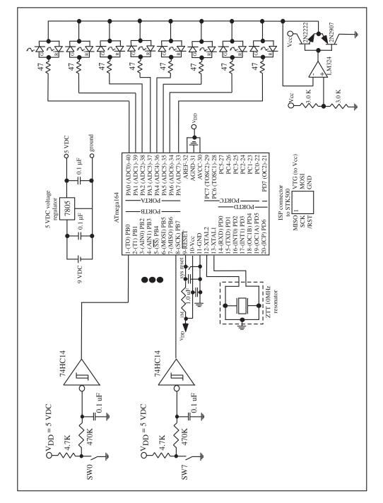
Figure 2.7: ATmega164 Testbench Hardware.
