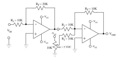
Figure 4.6: Operational amplifier implementation of the transducer interface design (TID) example circuit.
