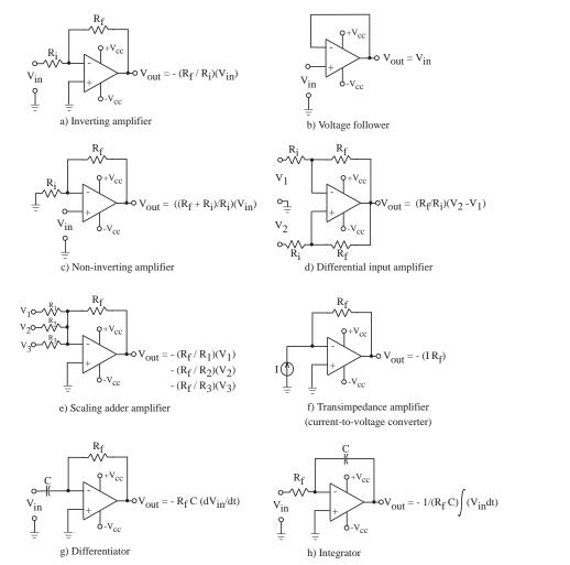
Figure 4.4: Classic operational amplifier configurations. Adapted from (L. Faulkenberry, 1982).
