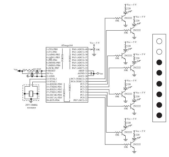
Figure 4.10: ADC with rain gage level indicator.
