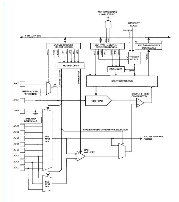
Figure 4.8: Atmel AVR ATmega164 ADC block diagram. (Figure used with permission of Atmel, Incorporated.)
