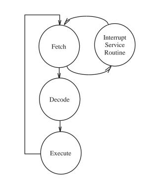
Figure 5.1: Microcontroller Interrupt Response.
