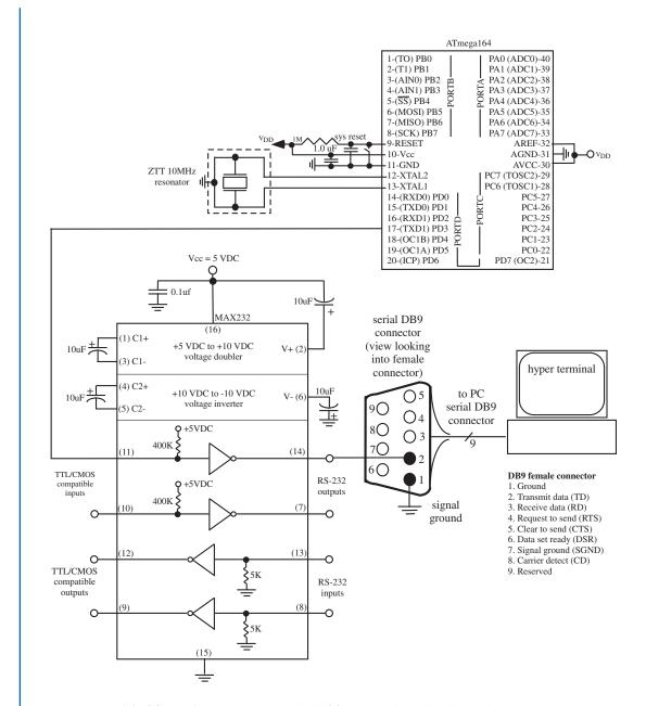
**Figure 3.8:** USART-to-PC communication link. This provides a handy method to print status statements from the microcontroller during code development.
