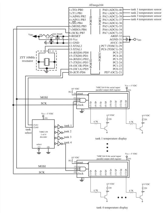
Figure 3.13: Aquarium tanks instrumented via SPI system.
