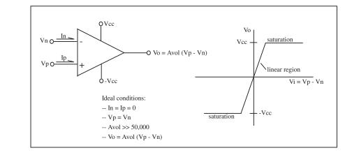
Figure 4.3: Ideal operational amplifier characteristics.
