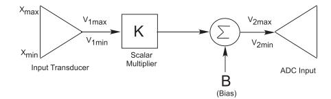
**Figure 4.2:** A block diagram of the signal conditioning for an analog-to-digital converter. The range of the sensor voltage output is mapped to the analog-to-digital converter input voltage range. The scalar multiplier maps the magnitudes of the two ranges and the bias voltage is used to align two limits.
