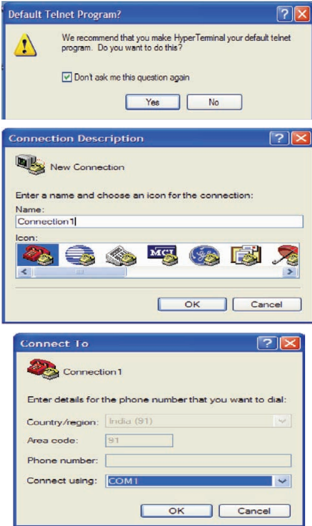
Fig. 4.2 Setting the necessary parameters of the HyperTerminal
