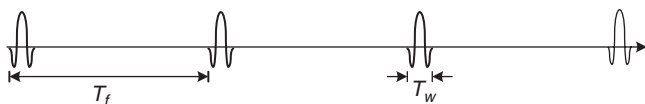
Figure 3.1 Pulse train with a low duty cycle, where T_f is pulse repetition time and T_w is pulse duration.
