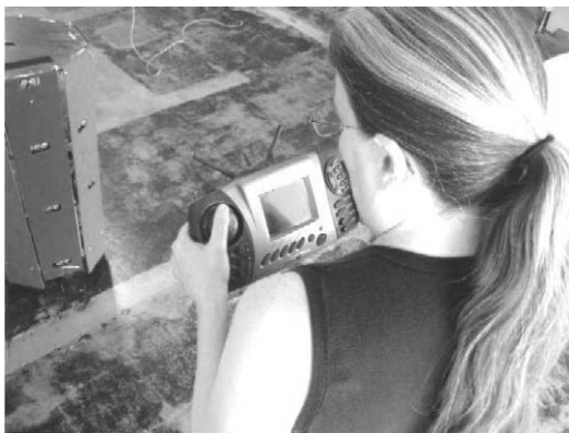
Fig. 7.1 In a teleoperated system, the human acts as a translator from the raw sensory images (provided by the video link) to a symbolic representation, and once a plan of action is determined, the operator translates that symbolic plan into a sensor/actuator based implementation using the joysticks and other controls. Shown here is one of the authors, using the teleoperation interface for a commercial robot.
