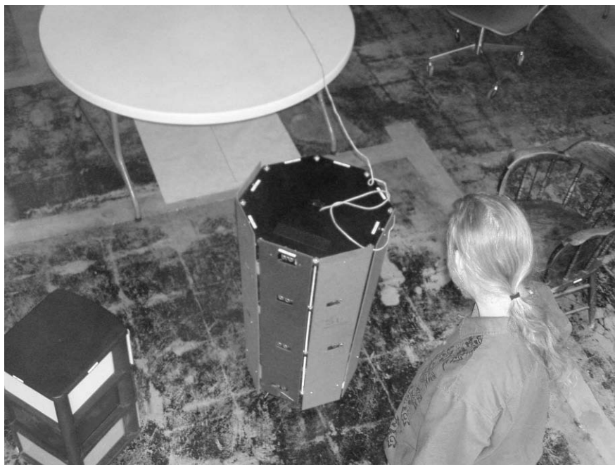
Fig. 12.6 This is the setup for the Prefference tests. The objects to be classified are groups around the robot with about 1m between their centroids (except the table which is at 1.5m). The objects are at 90 degree separation around the robot. One of the authors is the example of a person. Note the cable connected to the Robot. This is to enable the capture and analysis of the data generated by the test, the robot is running all software on its onboard processor.
