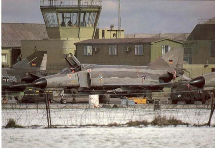
Parked on Binbrook's aircraft servicing pan (ASP), a Sidewinder AIM-9L-armed F-4F of JG 74, coded 37+80, is being readied for a sortie in the winter of 1985. The fairing under the nose houses the 20 mm M61A1 cannon introduced on the air force F-4E and also fitted to the Japanese F-4EJ
