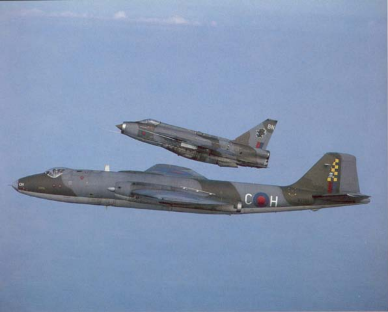
This Lightning F.6 from No 11 Sqn needs to be flown at a high angle of attack (AOA) to maintain formation on the somewhat slower Canberra (WT519) target facilities aircraft operated by No 100 Sqn
