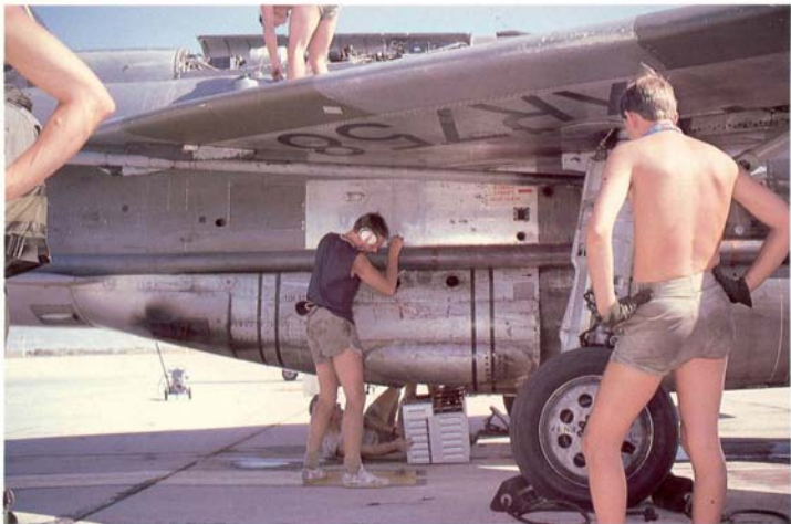
Armourers download the empty ammo tanks from a Lightning F.6 of No 11 Sqn during an operational turnround (OTR). The soot produced by departing shells is clearly visible downstream of the left-hand cannon port (extreme left)
