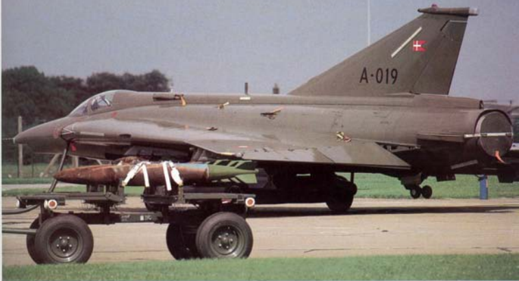
An immaculate A-35DX parked behind some rather less well-presented 500 lb (227 kg) low-drag bombs, or 'slicks'
