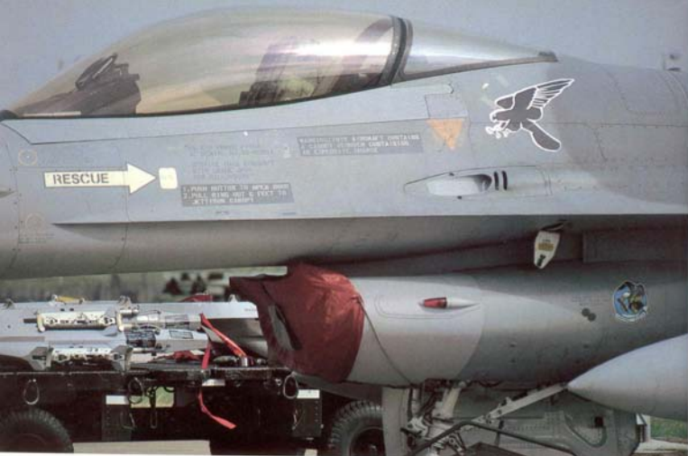
A Torrejon-based F-16 sporting a black 'Fighting Falcon' motif above the cannon port and blast deflector of its M61A1 Vulcan 20 mm cannon. This widely used six-barrel weapon can fire a maximum of 100 high-velocity shells per second. The average stoppage rate is just one round in 10,000
