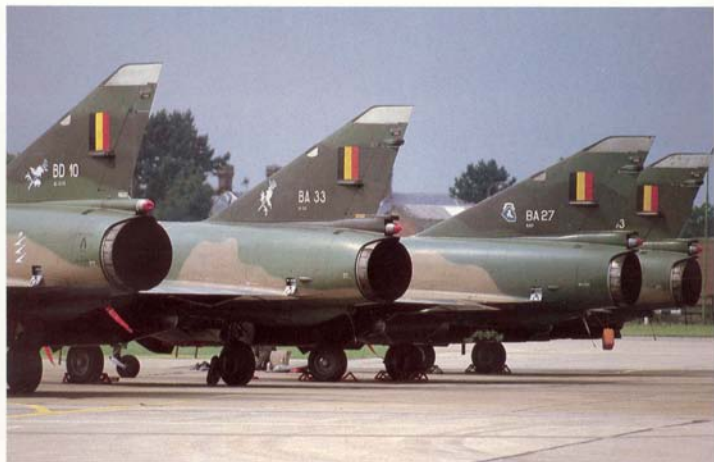
Mirage muscle: the 5 series is powered by the SNECMA Atar 9C single-shaft turbojet of 13,670 lb (6200 kg) thrust with afterburner. A parabrake is located in the fairing immediately above the engine nozzle
