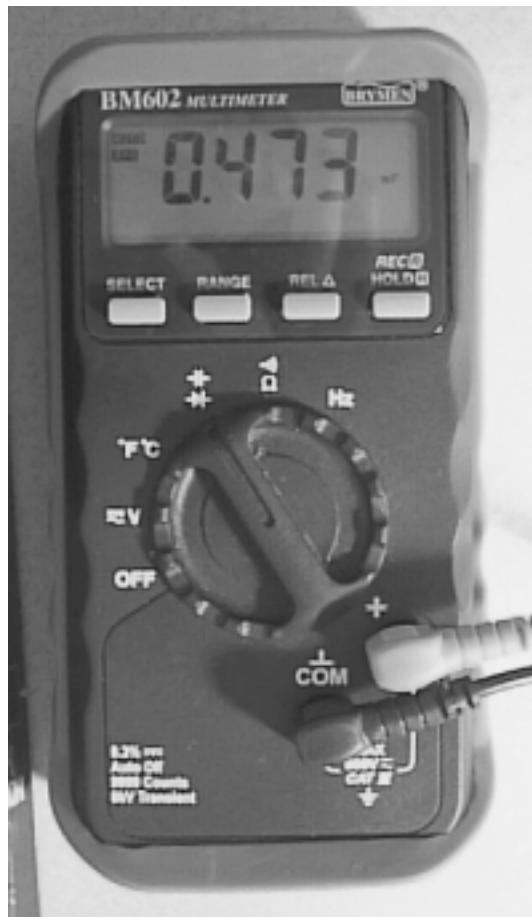
Figure 1.7 A multimeter is no longer a switched network of resistors and capacitors connected to a sensitive moving-coil microammeter. It still has the resistor and capacitor network, but now most of the switching is done by CMOS gates managed by a microcontroller.
