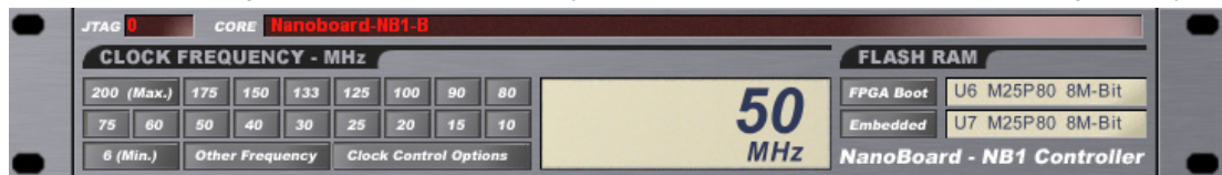
Figure 27. Use the NanoBoard controller to set the clock frequency and program the 2 flash RAM devices
