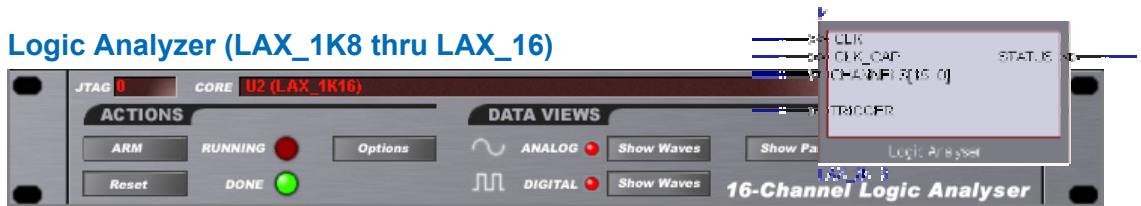
Figure 18. Logic analyzer instrument, with a logic analyzer component shown in the inset. Use the LAX to monitor multiple nets in the design, then display the results as a digital or an analog waveform.
