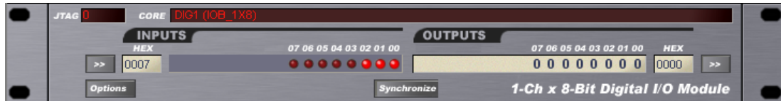
Figure 15. Digital IO module, used to monitor and control nodes in the design
